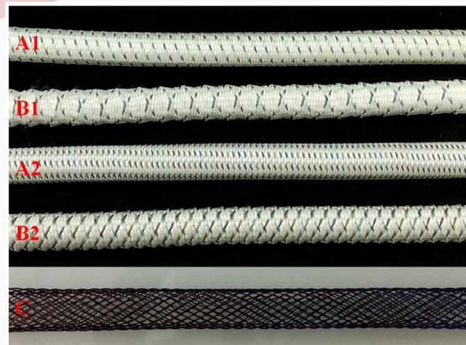
Fig. 1. Photographs of braided stent samples.
